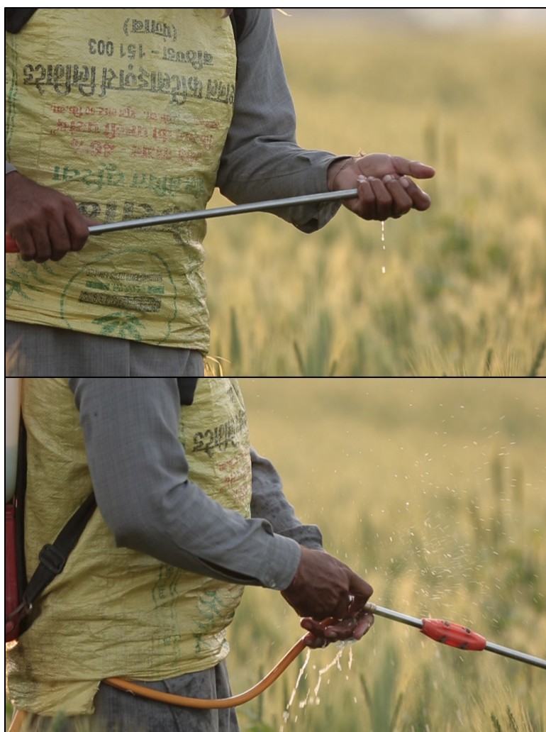
Picture 19: Poorly maintained, low-quality or otherwise faulty equipment exposes users to a greater risk of dermal contact. Lack of access to gloves exacerbates this contamination risk.
